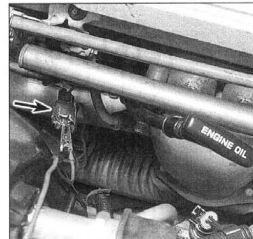
4.3 The cooling fan temperature switch is located in the right cylinder head just behind the engine oil dipstick. Unplug the electrical connector (arrow) and ground it and the fan should come on
