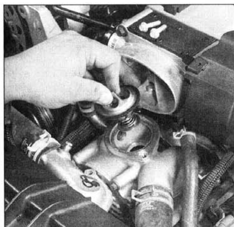
3.25 Note how the thermostat is installed, then remove the thermostat (the spring end points toward the engine)
