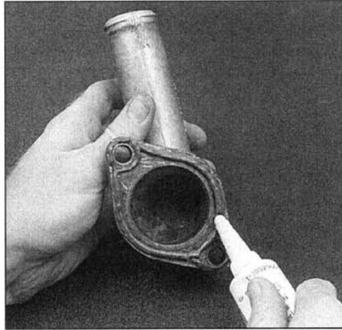
3.12 Apply a bead of silicone sealant on the mating surface of the thermostat housing
