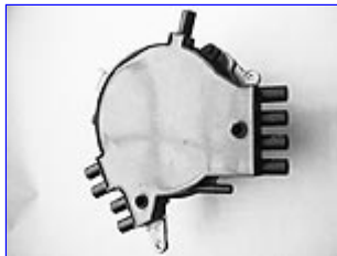
All Opti-Spark distributors use an encapsulated plastic distributor cap to protect the conductive ink that transfers the high-voltage to the spark plug wires from the rotor.
