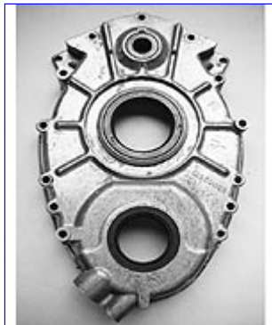
The OBD II-style case has a mounting boss for the crank sensor at the bottom of the casting.
