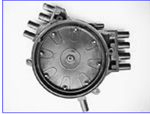
This is a later style, serviceable cap. It is identified by the small vent tube located in-between the secondary lead mounting points.
