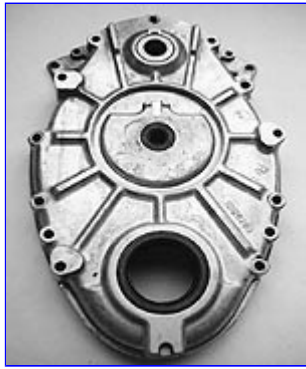
A first-generation timing cover. Note the small hole in the center to drive the distributor.
