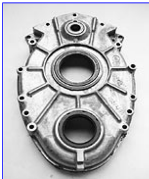
This timing case is for an interim year. It accepts the large drive mechanism but does not have a provision for the crank sensor.
