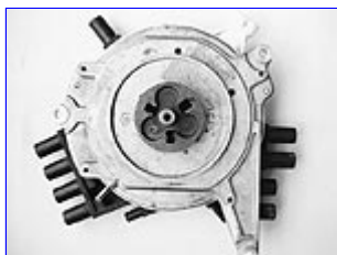
The revised version has a larger cam drive mechanism and an additional metal vent on the case of the distributor.
