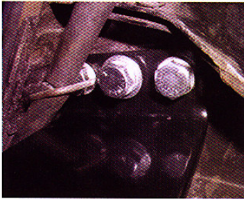
After installing all three threaded inserts, we found we could attach the parking-brake bracket by drilling an additional hole, bending the bracket slightly, and attaching it using a flat washer.
