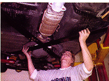
With the right-front-to-left-rear brace installed, we could lift the other half of the frame into place.
