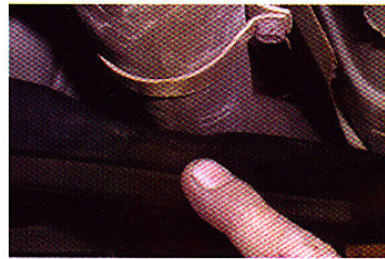
The cross frame is nicely made, with recesses to clear the exhaust system. As a result, we found the finished installation to be rattle-free.
