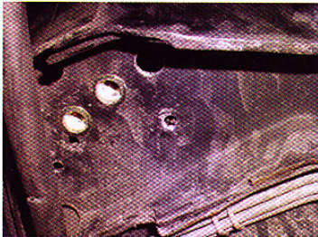
It's best to drill these holes and install the Nutserts one at a time, since there's a possibility the Nutserts will pull slightly off-center as they compress.
